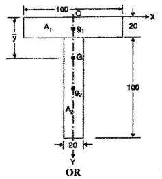
V. Calculate the moment of inertia of the I section shown in figure with respect to centroidal axis. XX and YY.
