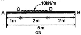
IX. Draw the shear force diagram and bending moment diagram of the beam shown in figure.
